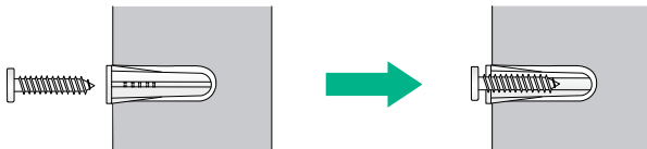
Figure 8 Driving a screw into a wall anchor
