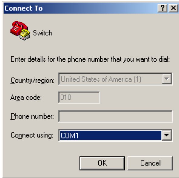
Figure 19 Setting the serial port used by the HyperTerminal connection
