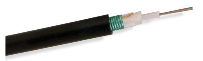
2 to 24 fibre OM1, OM2, OM3, OM4 multimode or OS1/OS2 (ITU-TG.652D) singlemode 250 µm single loose tube metallic armoured internal/external rodent resistant duct and direct burial/tunnel cable with E-glass strength members and Low Smoke Zero Halogen (LSZH) jacket.
